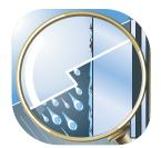
The photocatalytic action of Pilkington **Activ**<sup>™</sup> glass (upper) gradually breaks down and loosens organic dirt, while the hydrophilic action causes rain to sheet on the glass, leaving a clean exterior with minimal spotting or streaking.
