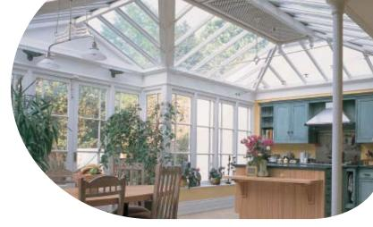
The proper application of Pilkington Activ<sup>TM</sup> is with the Pilkington Activ<sup>TM</sup> surface glazed to the exterior of a building (#1 surface) in either a monolithic or Insulating Glass Unit (IGU). The Pilkington Activ<sup>TM</sup> surface requires several days exposure to daylight to be activated.
